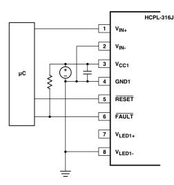
Figure 68. Typical input configuration, noninverting.
