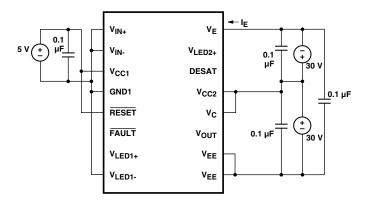
Figure 61. I<sub>EL</sub> test circuit.
