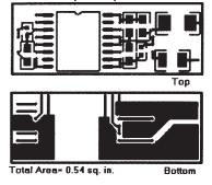
Maximum Components placed on two sides
