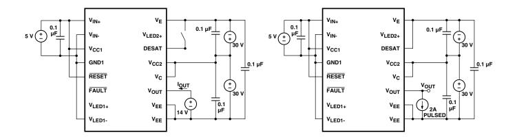
Figure 34. I<sub>OLF</sub> test circuit.
