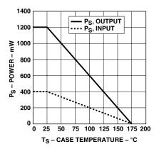
Figure 2. Dependence of safety limiting values on temperature.
