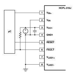
Figure 70. Local shutdown, local reset configuration.
