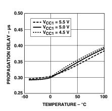
Figure 18. Propagation delay vs. supply voltage.
