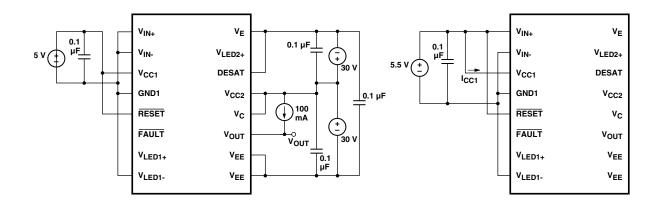
Figure 36. V<sub>OL</sub> test circuit.
