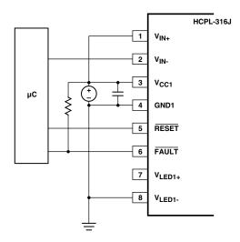
Figure 69. Typical Input Configuration, Inverting.
