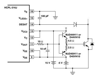
Figure 75. Current buffer for increased drive current.
