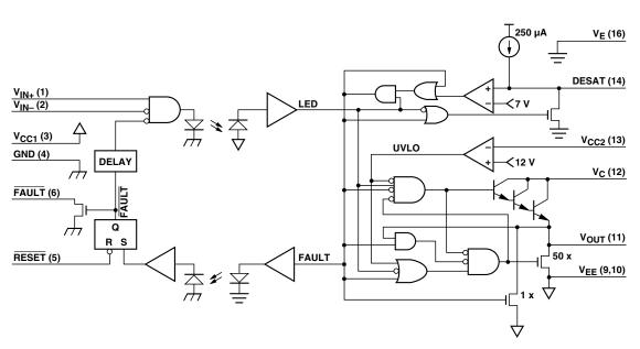
Figure 64. Behavioral circuit schematic.
