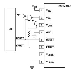
Figure 73c. Safe hardware reset for inverting input configuration.
