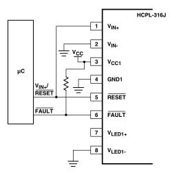
Figure 73a. Safe hardware reset for noninverting input configuration (automatically resets for every V<sub>IN+</sub> input).
