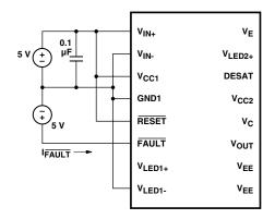
Figure 30. IFAULTL test circuit.
