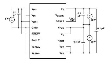
Figure 40. I<sub>CC2L</sub> test circuit.
