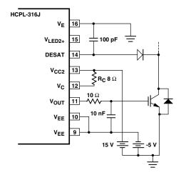
Figure 74. Use of R<sub>C</sub> to further limit I<sub>ON.PEAK</sub>.
