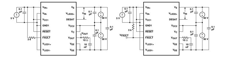
Figure 46. t<sub>DESAT(10%)</sub> test circuit.
