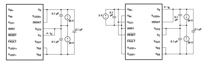
Figure 59. I<sub>CL</sub> test circuit.
