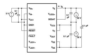
Figure 80. Minimum LED Skew for Zero Dead Time.
