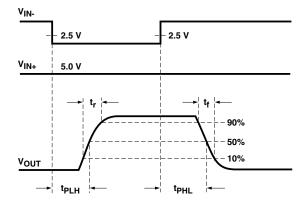
Figure 54. V<sub>OUT</sub> propagation delay waveforms, noninverting configuration.
