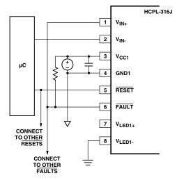
Figure 71. Global-shutdown, global reset configuration.
