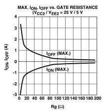
Figure 76. Typical peak  $I_{\rm ON}$  and  $I_{\rm OFF}$  currents vs. Rg (for HCPL-316J output driving an IGBT rated at 600 V/100 A.
