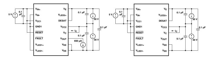
Figure 57. I<sub>CH</sub> test circuit.
