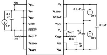
Figure 44. DESAT threshold test circuit.
