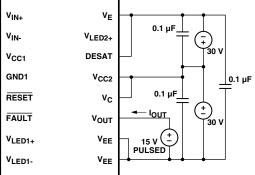
Figure 32. I<sub>OH</sub> pulsed test circuit.
