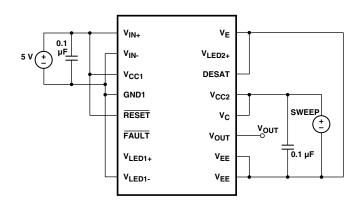
Figure 42. I<sub>DSCHG</sub> test circuit.
