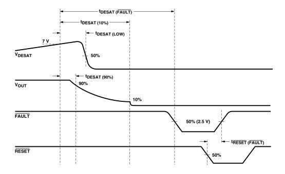
Figure 56. Desat, V<sub>OUT</sub>, fault, reset delay waveforms.
